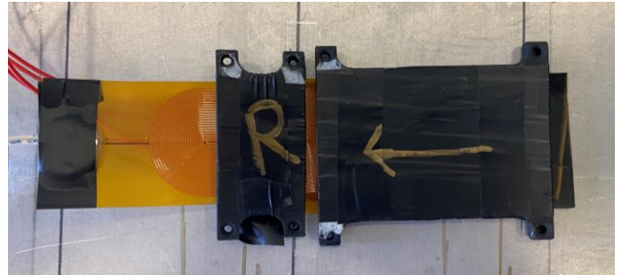
FIGURE 10: PROTOTYPE UNIDIRECTIONAL TRANSMITTER AND RECEIVER TRANSDUCER SETUP.
