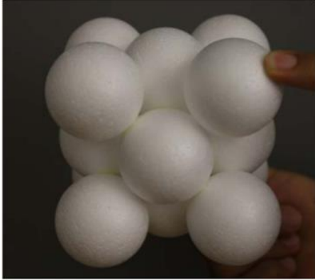
Fig. 2. 15. Crystal lattice Face-Centered-Cubic (FCC) model of the austenite \gamma -phase [105].
