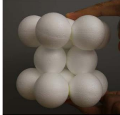
Fig. 2. 16. Cristal lattice Hexagonal-Close-Packed (HCP) model of the martensite \epsilon -phase [105].
