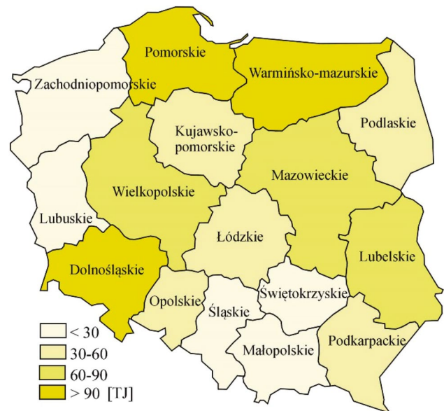
Fig. 12 Distribution of the amount of energy that can be obtained annually from PV panels in closed municipal landfills in Poland (own study)
