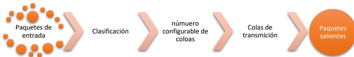
**Figura 2.***Principio de Operación de WFQ*
