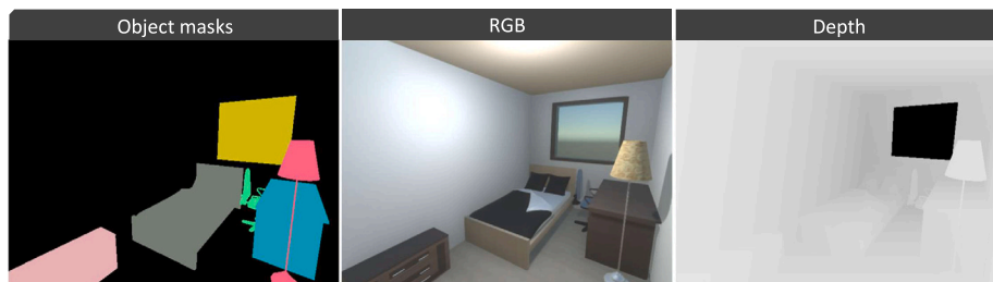
Fig. 6. Images returned by the Smart Camera . On the left, image of instance segmentation masks, where each color represents a different object. In the middle, the RGB intensity image. On the right, the depth image.
