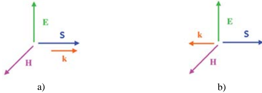
Fig. 1-5 Poynting vector S and phase vector k : a) going in the same direction, and b) going on opposite directions 2 .
