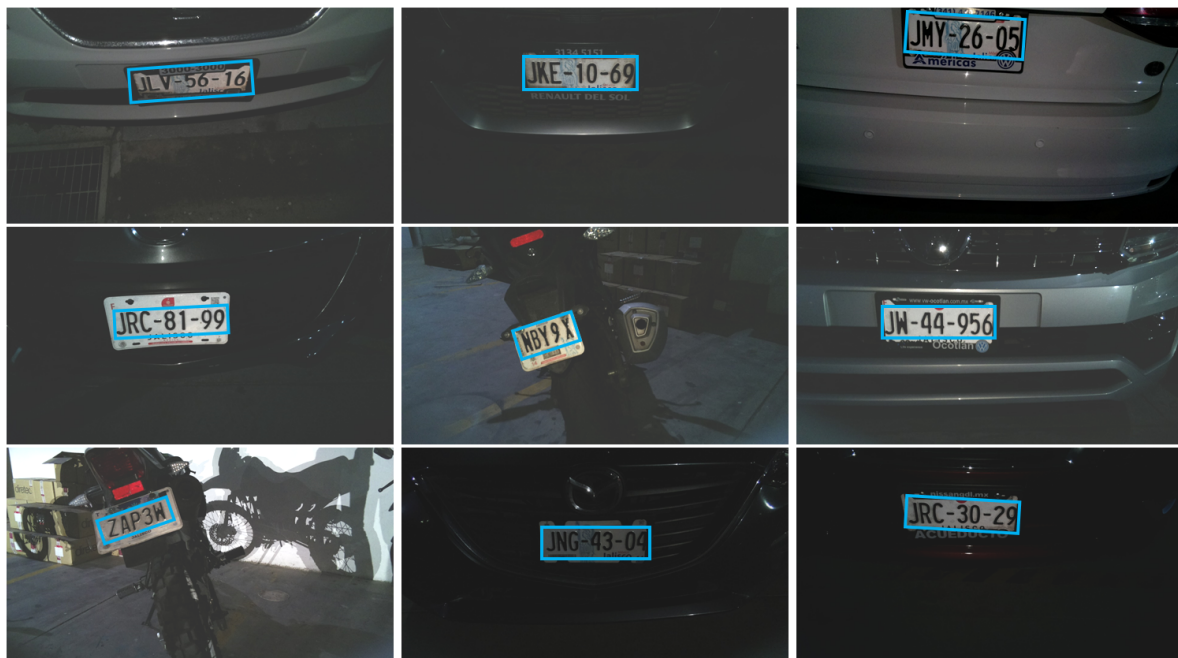
Figure 21. License plate identification results for different environmental conditions.
