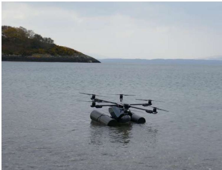
FIGURE 8 | TD7 water-landable UAV under trial on a near calm and sheltered embayment at Dunstaffnage Peninsula, Argyll, Scotland.
