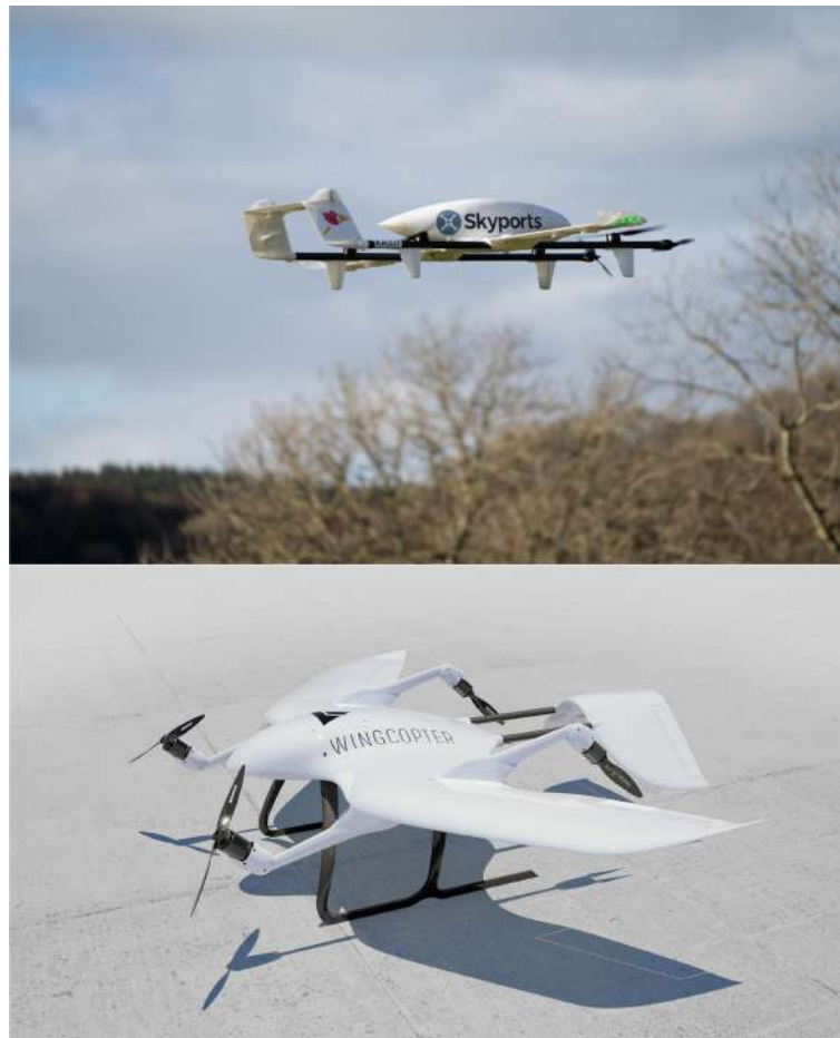
FIGURE 9 | The Skyports aircraft (Wingcopter VTOL winged aircraft) showing the swivel-mounted forward motors in take-off/landing mode. The under-slung payload 'pod' is visible. Reproduced with permission of Wingcopter.
