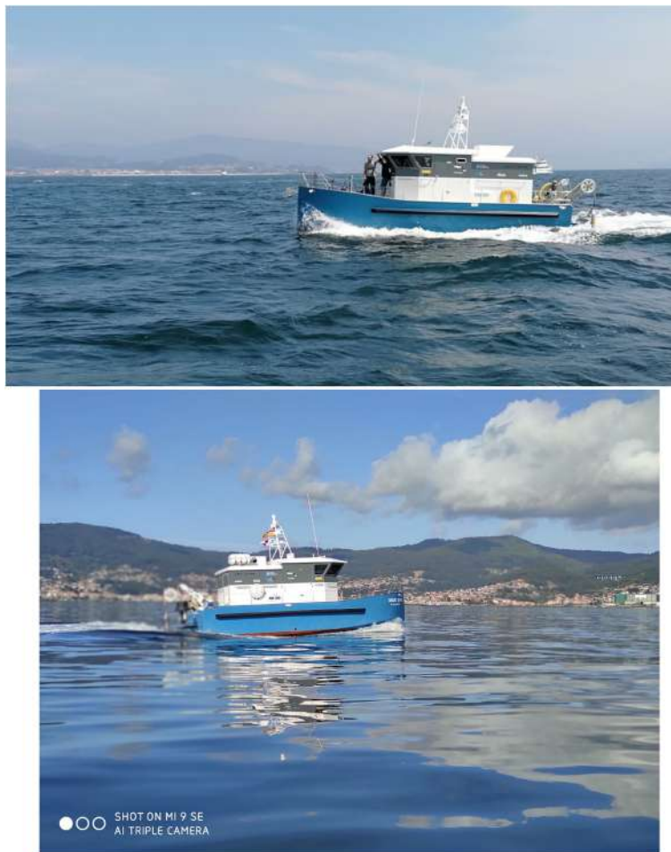
FIGURE 11 | The USV Mar II prototype, developed in the Galician CIVIL UAV Initiative for Automatic oceanographic sampling, operating in the Galician Rias in manned and unmanned mode. Pictures provided by GAIN, Xunta de Galicia, Spain.
