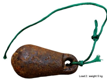
Load 2: weight 5 kg Standard iron weight in the polypropylene line, 8 mm \varnothing , y 25 m length
