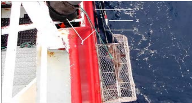
Figure 6 Cradle hoisted just above surface to cut snood.
