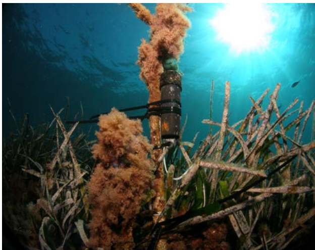
Figure 3. Underwater sensor for the continuous measurement of water temperature in Grosa Island, Spain (5m depth). Photo credit: Juan Manuel Ruíz.
