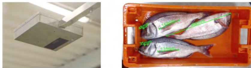
Figure 1. On the left: Scanner mounted above a scale; on the right: image acquired by the scanner, with some measures between 3D points.
