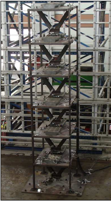
Figure 2-6 Photo of the 6-story structure and its instrumentation. AX are the accelerometers.
