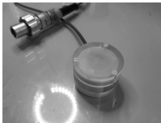
FIGURE 1 UTIC1 prototype with a distance between electrodes of 0.27 mm
