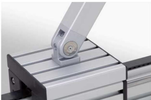
Ball-Bearing Hinge 8 40x40 is a fastening element for profiles that allows swivelling around 180°. The construction features a swivel axis with dual ball-bearing and guarantees high strength and low wear in continuous operation.
