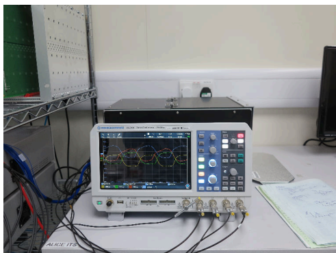
(a) An oscilloscope sits in front of the HIC test box in the LSDC. The oscilloscope is used for the DCTRL test.
