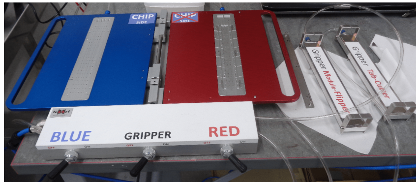
Figure 5.11: Module flipper machine. Each HIC is flipped from silicon side down to silicon side up using a system of rotating vacuum grippers. The ‘Gripper Module-Flipper’ and ‘Gripper Tab-Cutter’ seen on the right are used to move the HIC from the module flipper to the tab-cutter.
