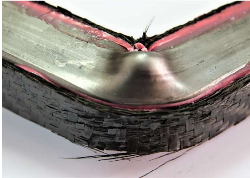
Figure 5.14: Composite failure in UD25x2 due to normal bending stress in the lower portion of the collapsed zone in top and bottom reinforcements.
