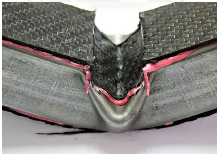
Figure 5.15: Indentation failure in UD50x2 shapes.
