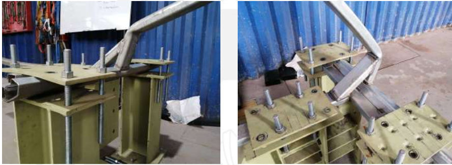
Figure 3.9: Bending tests performed on the structural joint of a bus. Note that the bending collapse is the dominant failure mode.
