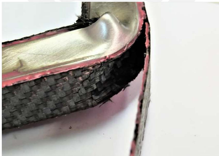
Figure 5.13: Mode II failure scenario found with top and bottom reinforcements of UD25x2. This is the most commonly found failure scenario.
