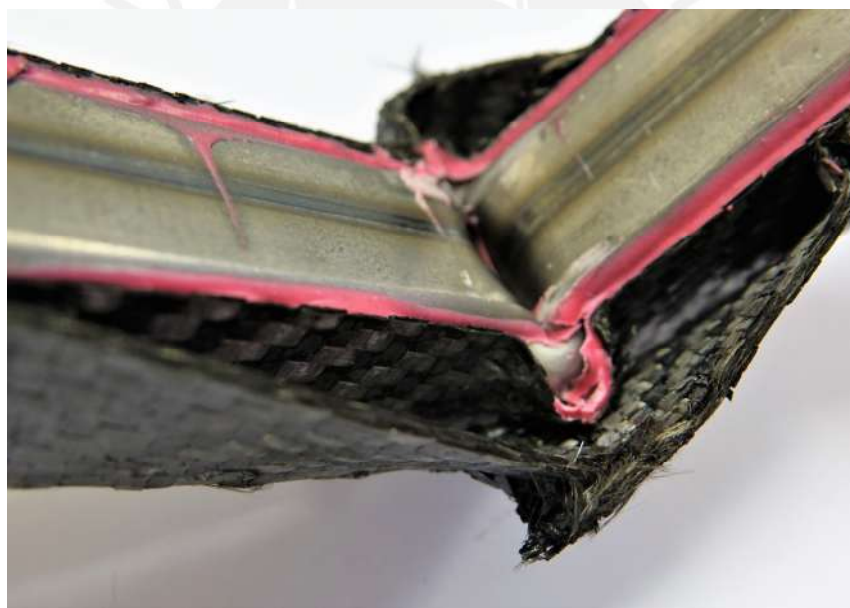
Figure 5.17: Specimen with LR reinforcement, showing that the inner layers of CFRP are still attached to the steel tube.
