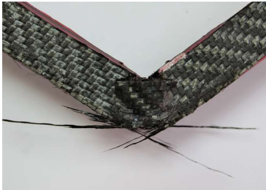
Figure 5.16: Composite failure in the exterior layers of the LR reinforcement.
