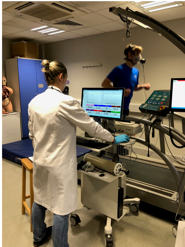
Figure 3.2 Assessment of \dot{V}O_{2max} . A participant performing the \dot{V}O_{2max} test on a motorized treadmill (HP Cosmos Mercury 4.0)
