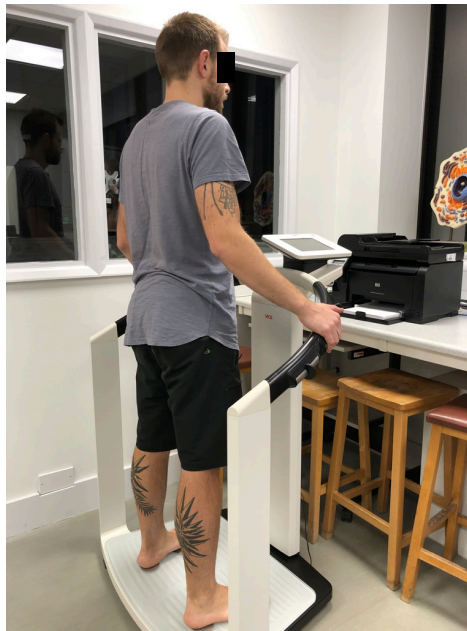
Figure 3.1 Assessment of body composition using SECA (Seca® mBCA 514 Medical Body Composition Analyzer). A participant standing in bare feet on the body composition analyser during assessment
