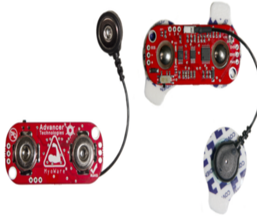
Figura 2.7: Sensor Myoware de 1 canal [7].
