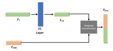
**Figure 5.** The weighted concatenation method for fusing CNN features  $F_{CNN}$  and traditional handcrafted features  $F_T$ . First, a fully-connected layer is adopted to ensure that the dimension of  $F_T$ is unified with that of  $F_{CNN}$ . Then, we set two learnable weight parameters  $\alpha$  and  $\beta$  to reveal the importance of different features. Finally, the two features are fused by the concatenation operation.
