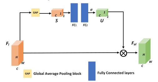
**Figure 3.** The operation process of the SE-Net. The channel descriptors are first generated by global average pooling, then the attention values are calculated by the fully-connected layers. Finally, the channel-refined features can be calculated by performing channel-wise multiplication.  $\otimes$  represents the channel-wise multiplication operation and  $\sigma$  denotes the sigmoid function.
