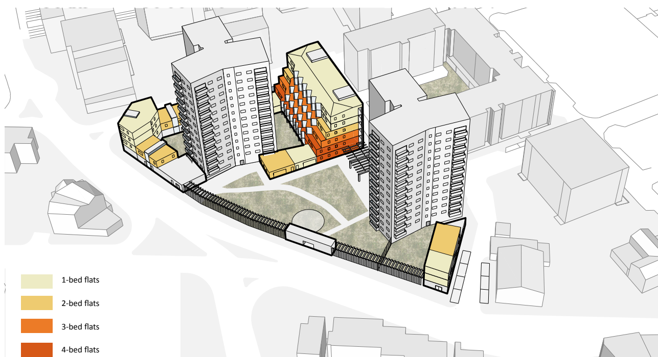
Figure 5.4: Provision of new infill homes.
