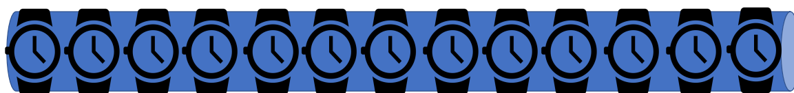
Figure 3.2.7. Schematic drawing of all the Actiwatches mounted on a solid board for inter-device reliability measures. Diagram not to scale.
