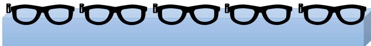
Figure 1. Schematic drawing of the Clouclips mounted on spectacle frames attached to a solid, portable board for inter-device reliability measures. Diagram not to scale.
