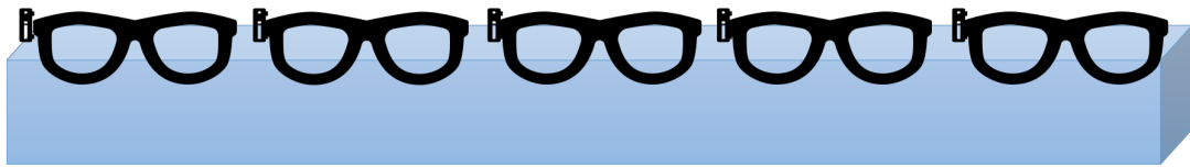
Figure 3.2.8. Schematic drawing of the Clouclips mounted on spectacle frames attached to a solid, portable board for inter-device reliability measures. Diagram not to scale.
