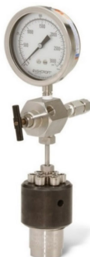
Fig. 3.2. Hydrothermal Parr reactor (Parr Instruments) used for \text{BiVO}_4 synthesis
