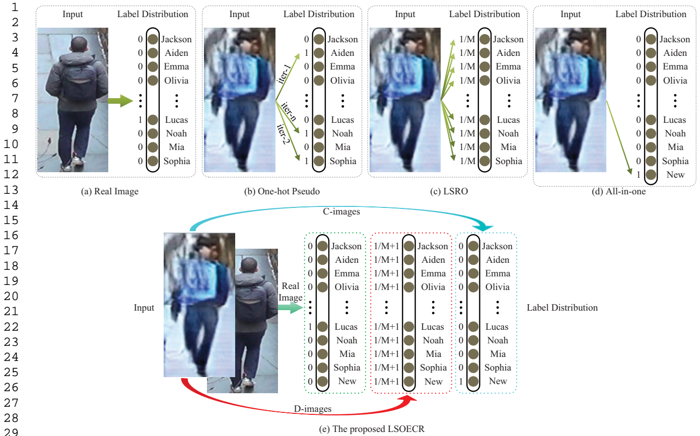
Fig. 4 The label distributions of a real sample and a generated sample. The real data (a) is assigned the ground-truth label, i.e., the classical label distribution. For a generated sample, one-hot (b) assigns each unmarked sample a dynamic class label in each training epoch. LSRO (c) uses a uniform label distribution. All-in-one (d) treats all unmarked images belong to a new class. (e) the label distribution proposed in this work.
