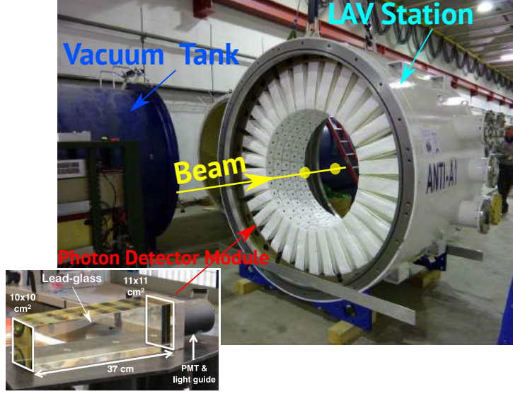
Figure 3.12: Annotated photograph of a LAV station during its installation and photon detector module during construction (adapted from [211] and [200] respectively).
