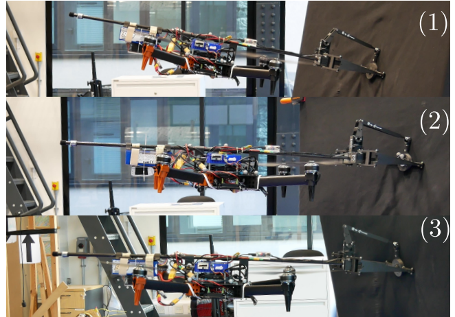
Fig. 1: Stable orthogonal physical interaction on an inclined and/or angled target surface for: (1) an inclined target requiring the system to pitch; (2) an angled target requiring the system to reorient in yaw; (3) an inclined and angled target requiring the system to both pitch and reorient in yaw. When the target is angled, the flying base yaw reorientation strategy is utilized.
