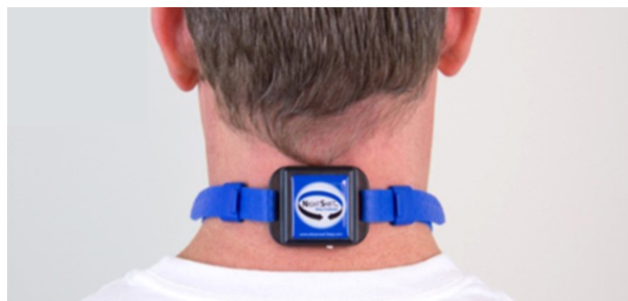
Figure 2.5: Vibrotactile PT device, The Night Shift™ (Advanced Brain Monitoring, Carlsbad, CA, USA)
