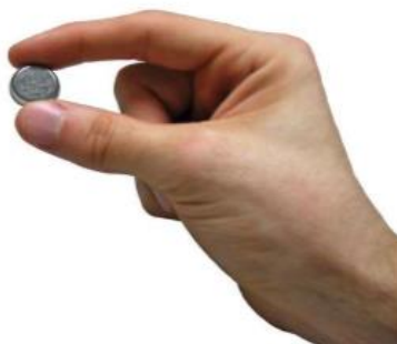
Figure. 2. Skin temperature data logger.
