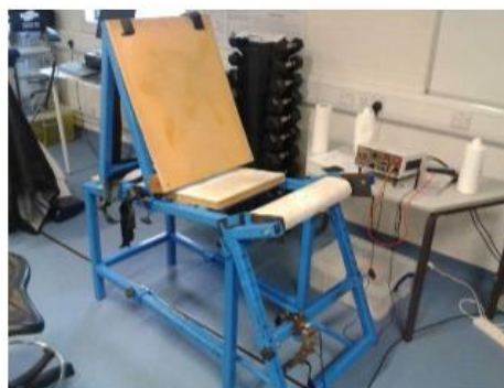
Figure. 3. Custom built isometric strength chair.
