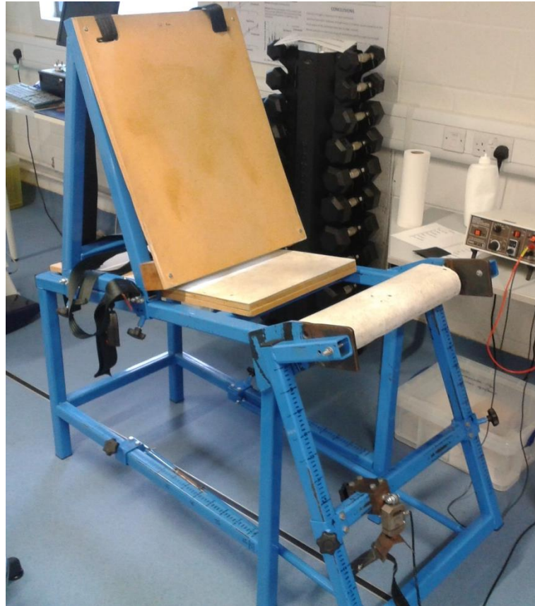
Figure. 3.1. Custom-built isometric strength testing chair used to perform unilateral contractions of the knee extensors. The same testing rig was used in all experimental chapters.
