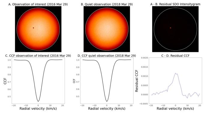
Figure 1. Residual CCF ( $\triangle$ CCFs) construction. Top row: SDO/HMI intensity grams; bottom row: CCFs from HARPS-N Solar Telescope observations. Panels (a) and (c) are from a period of relatively large solar activity, while panels (b) and (d) are from observations of the quiet Sun. To highlight differences in shape between CCFs, in the right column we subtract a quiet observation (B/D) from the observation of interest (A/C).
