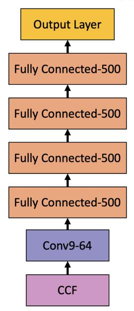
**Figure 6.** The architecture of our best-performing neural network model. Convolutional layers are denoted conv  $\langle kernel \ size \rangle - \langle number \ of \ feature \ maps \rangle$ , and fully connected layers are denoted Fully Connected –  $\langle number \ of \ units \rangle$ .
