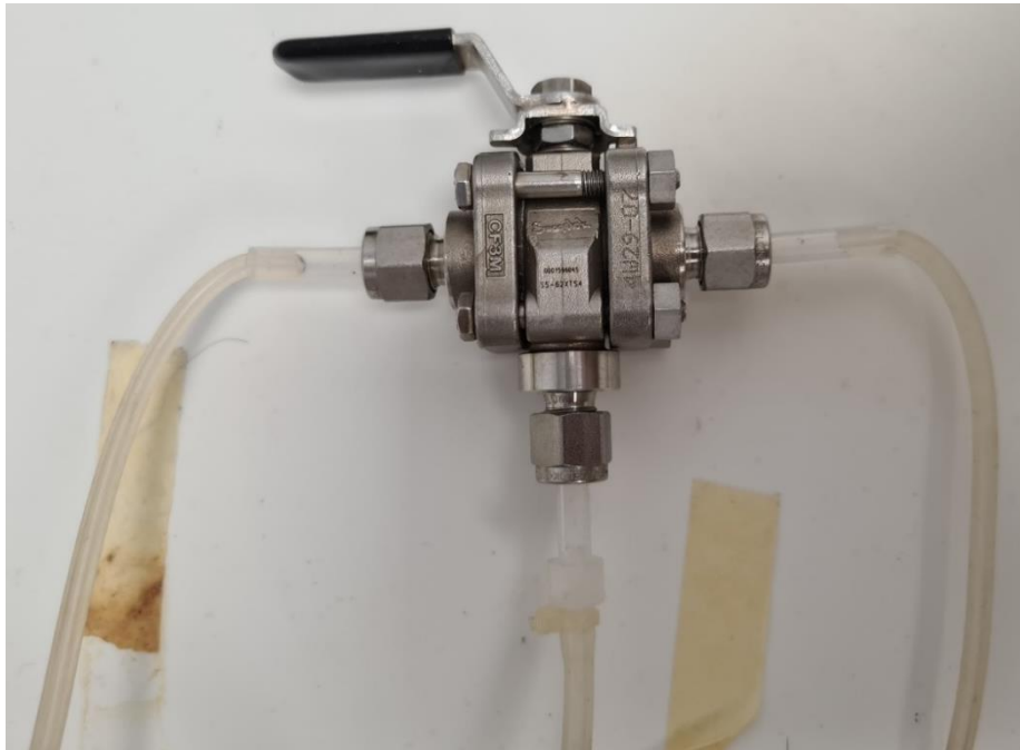
Figure 7: Three-way connector enabling a sterile switch from continuous pumping of 12 C glucose ASM to 13 C-labelled ASM.
