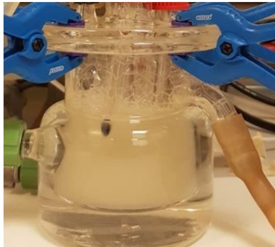
Figure 30: 'MKII' bioreactor system featuring excessive foaming. Due to the wall mounted efflux port, excessive foaming could result in only foam being removed from the culture, leading to a more fed-batch style of growth.
