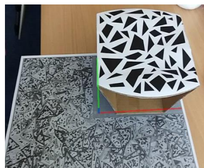
(b) Calibration of an irregularly patterned object
