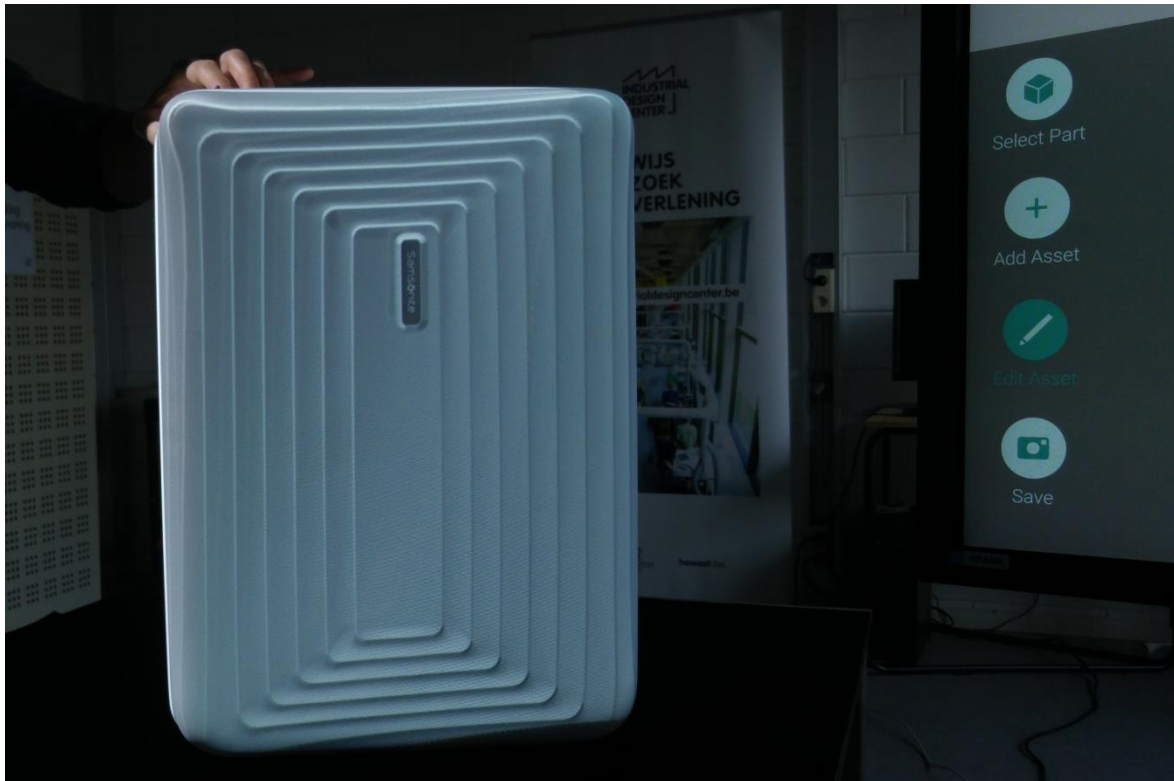
Figure 95. Samsonite Neopulse model physical prototype with SAR projected texture during the calibration phase. The vertical multi-touch screen shown in Figure 93 can be seen in the background on the right of the image. The interface buttons are visible showing options such as “select part” and “add asset”.
