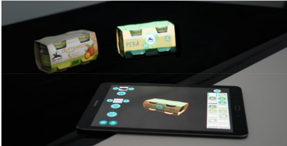
Figure 75. A real life object (left) next to a physical model with a digital overlay (right) the tablet shows the interface used to control the SAR projection (Becattini et al., 2018)
