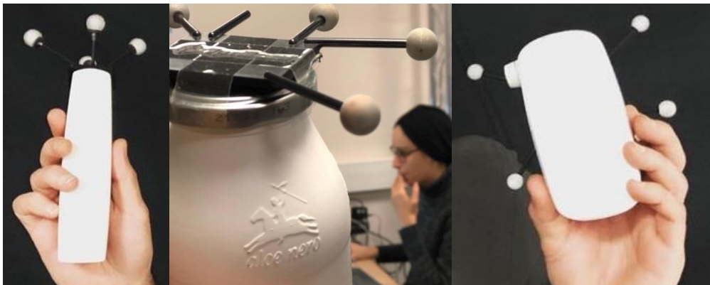
Figure 38. Three mixed prototypes. All have been painted matte white with paint and have been fitted with a “constellation” of IR trackers (SPARK Consortium, 2018d, 2019a)
