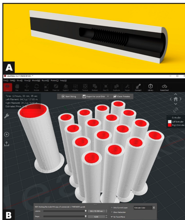
Figure 3. (A) Cross-sectional CAD view of the AM electrodes. (B) Screen capture of the IdeaMaker generated .GCODE file of 16 AM electrodes.
