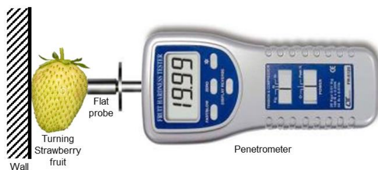
Fig. 2.2. Penetrometer used for measuring fruit softness. A penetrometer with a 5-mm flat probe was used for measuring the fruit softness. The probe was pushed against the fruit supported by a hard stationary wall behind. Readings (in newtons) were taken of the force required to cause 20% (of the total fruit diameter) surface deformation.
