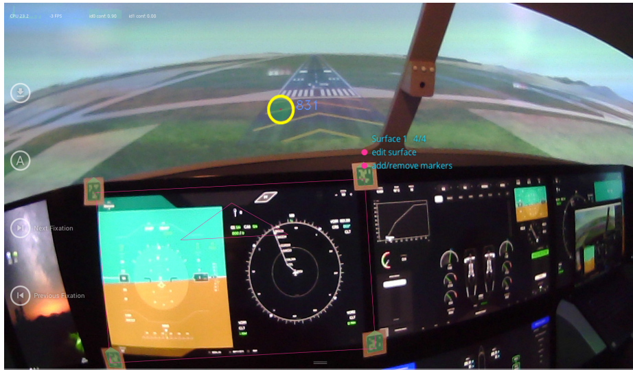
Fig. 3. Pilot's perspective and example fixation (here: the pilot is looking on the outside of the window).
