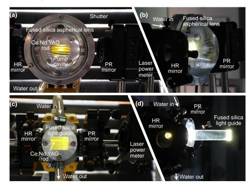
**Figure 4.** Photographs of the front view (**a**,**c**) and side view (**b**,**d**) of the Ce:Nd:YAG solar laser heads using the fused silica aspherical lens (**a**,**b**) and the fused silica light guide (**c**,**d**). PR: partial reflection; HR: high reflection.
