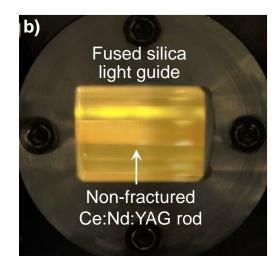
**Figure 7.** Photograph of the Ce:Nd:YAG laser rods on the laser heads with the fused liquid fused liquid aspheric lens (**a**) and rectangular light guide (**b**) after the solar laser experiments. The fracture on the Ce:Nd:YAG laser rod using the aspheric lens is visible on its central region.
