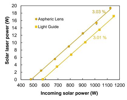
**Figure 6.** Solar laser power as a function of the incoming solar power of the Ce:Nd:YAG side-pumped solar lasers with the aspherical lens and the light guide secondary concentrators. Error bars, when not hidden by symbols, are for standard deviation.
