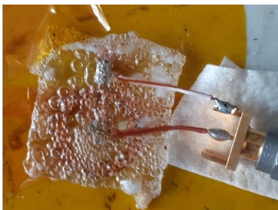
Figure 31 – Aspect of the sensor with the electrolyte after 2 weeks and 3 measurements with temperature.
