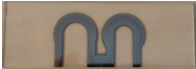
Figure 7 - Sputtered Resistors on glass microscope slide
