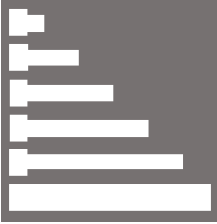
Figure A. 1- Shadow mask used to fabricate the MIM capacitors. (Area=2.5cm 2 )
