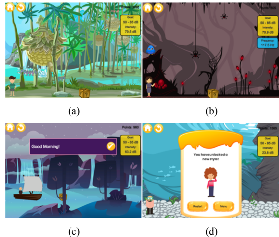
Figure 1. The game in the (a) sustained vowel mode, the (b) sustained vowel with frequency variations mode, and the (c) functional phrases mode. The yellow and blue boxes show information about the vocal intensity and vocal frequency, respectively. (d) Several scenarios and characters are available and can be unlocked through a points and rewards system.
