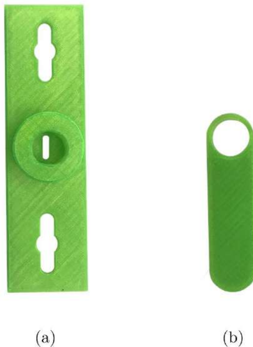
Figure 1: Designed structures for the present protocol: (a) finger's support; (b) horizontal tab.
