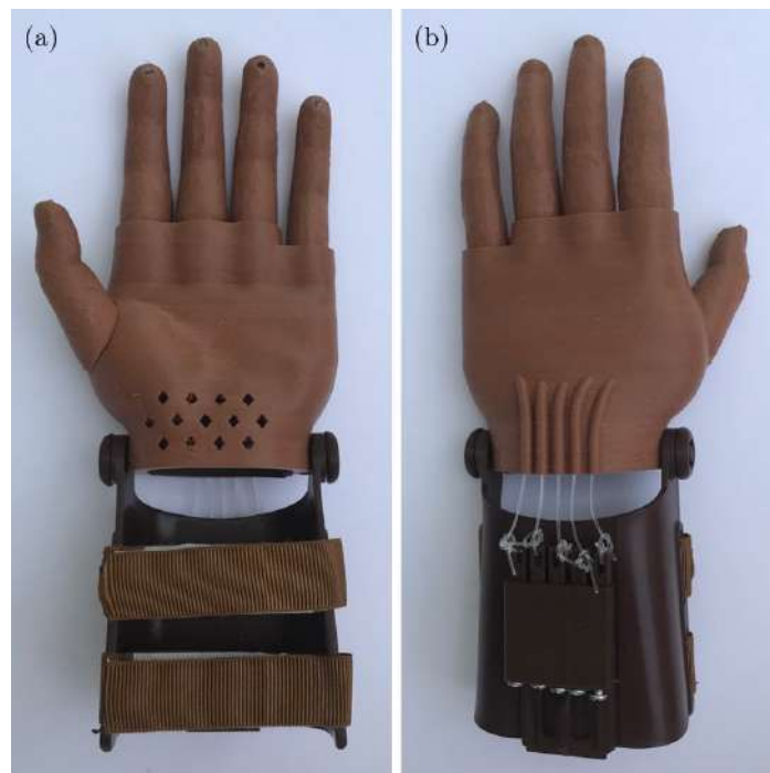
Figure 6.49: Second developed prosthesis: this prosthesis was developed in order to find out if the filament colour had some influence in its printing quality and consequently, in the prosthesis functionality; (a) anterior view; (b) posterior view.
