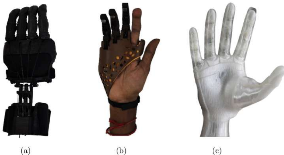
Figure 4.7: Examples of other prostheses with components made of flexible materials (adapted): (a) body-powered prosthesis developed by J. Corveira [79]; (b) cosmetic prosthesis for finger replacement developed by R. Alturkistani et al. ; (c) X-Limb, a robotic hand prosthesis [82].
