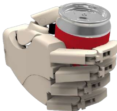
Figure 4.3: Nazree's Prosthetic Hand [78].
