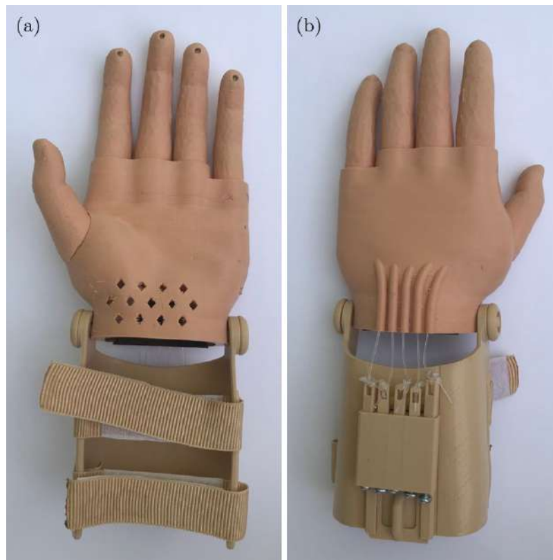
Figure 6.47: First developed prosthesis: this is the main prosthesis, that was printed with nude filaments to match the skin colour of the child; (a) anterior view; (b) posterior view.
