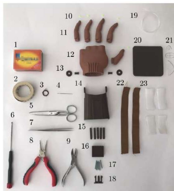
Figure 5.18: Prosthesis' components and needed tools for its assembly: 1. Matchsticks; 2. Measuring tape; 3. Thread; 4. Needle; 5. Scissors; 6. Phillips head screwdriver; 7. Fine tip tweezers; 8. Round nose plier; 9. Cutting plier; 10. Rings; 11. Fingers; 12. Metacarpal region; 13. Thermo pins and caps; 14. Gauntlet; 15. Tensioner pins; 16. Tensioner block; 17. M3 screws; 18. Retention clip; 19. Guitar strings; 20. Adhesive foam; 21. Paper moulds; 22. Grosgrain ribbons; 23. Velcro tape.
