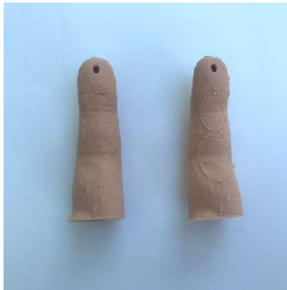
Figure 6.22: Printing results of the finger prototypes with thinner chambers' external walls: seventh prototypes with 0.6 mm (left) and with 0.3 mm wall thickness (right).
