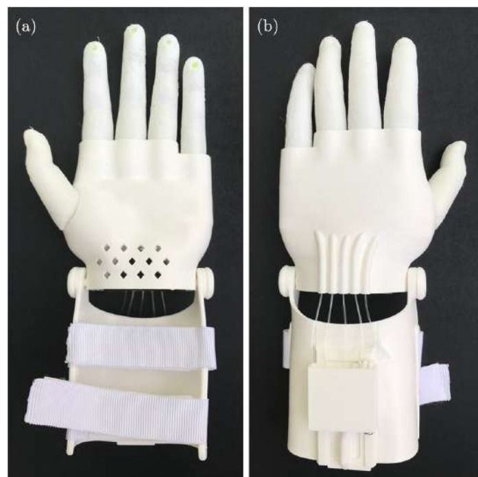
Figure 6.50: Third developed prosthesis: this prosthesis was developed in order to evaluate the hypothetical functionality of the third and second prostheses, by eliminating the hardness difference between the metacarpal region and the gauntlet. It also presents a different tensioning mechanism, a whippetree system; (a) anterior view; (b) posterior view.
