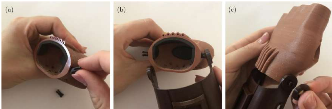
Figure 5.21: Connection between the gauntlet and the metacarpal region structure: (a) fitting of the thermo pins in the metacarpal region structure; (b) fitting of the gauntlet in the thermo pins; (c) introduction of the wrist pin caps.
