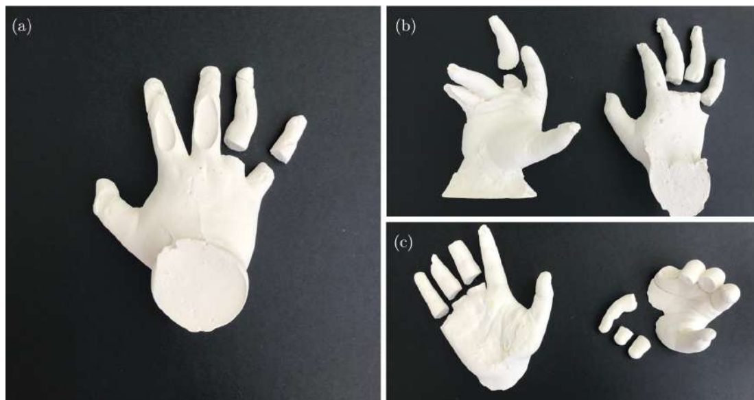
Figure 6.2: Body casting failures: (a) first body casting attempt with two broken fingers and presence of air bubbles; (b) second body casting attempt where it was made more than one replica. Both present air bubbles, broken fingers and poor quality; (c) third body casting attempt made by the child's mother with broken fingers.
