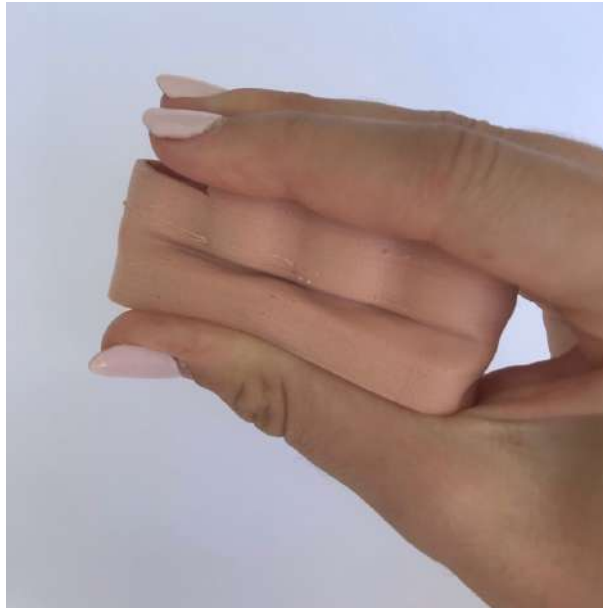
Figure 6.32: Flexion of the third prototype of the metacarpal region: in order to avoid more material waste, only part of the prototype was printed.
