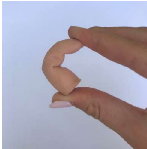
Figure 6.20: Flexing of the finger prototype with no phalanges: this index model was designed without phalanges to evaluate if the reduction of printing walls would influence their performance. However, it revealed worse results, especially in the middle phalanx area.
