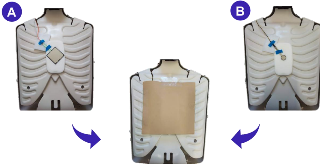
Figure 4.8. Pressure sensors arrangements on the manikin: (A) Interlink FSR 406 and (B) Interlink FSR 402.
