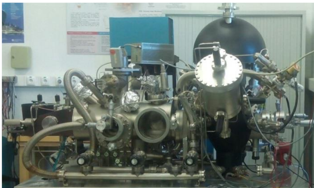
Figure 3.1 – Picture of the Kratos XSAM 800 system, taken in the surface science lab of CEFITEC.
