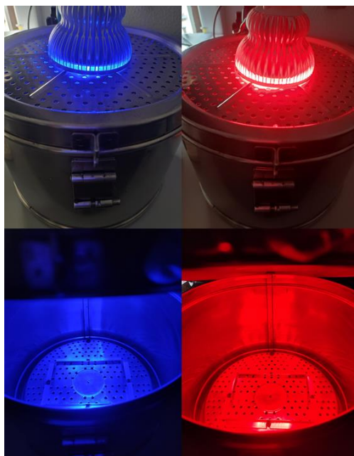
Figure 4.13: Photo of the system used for the cells irradiation exemplifying the blue light and the red light emissions.
