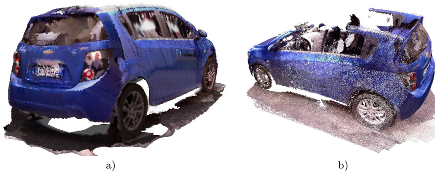
Fig. 11 Reconstruction of a Chrevolet Aveo (from 1300frames). a) View from the back; b) side view with the roof purposely removed in order to show the interior.
