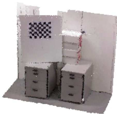
Fig. 9 Reconstruction of a simple office scene (from 100 frames).
