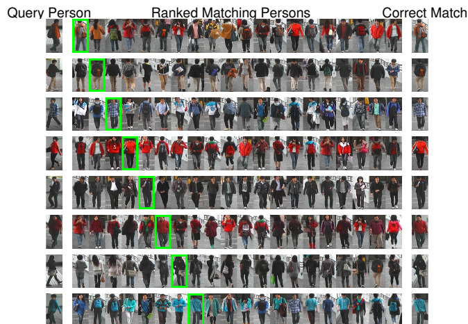
Fig. 6. Qualitative performance of MuRE (LFDA-KISSME-LADF) on the CUHK02 dataset. In the first column 8 query persons are shown. The next 20 images per row represent the ranked matching persons. The correct match (also shown in the last column) is highlighted in green.
