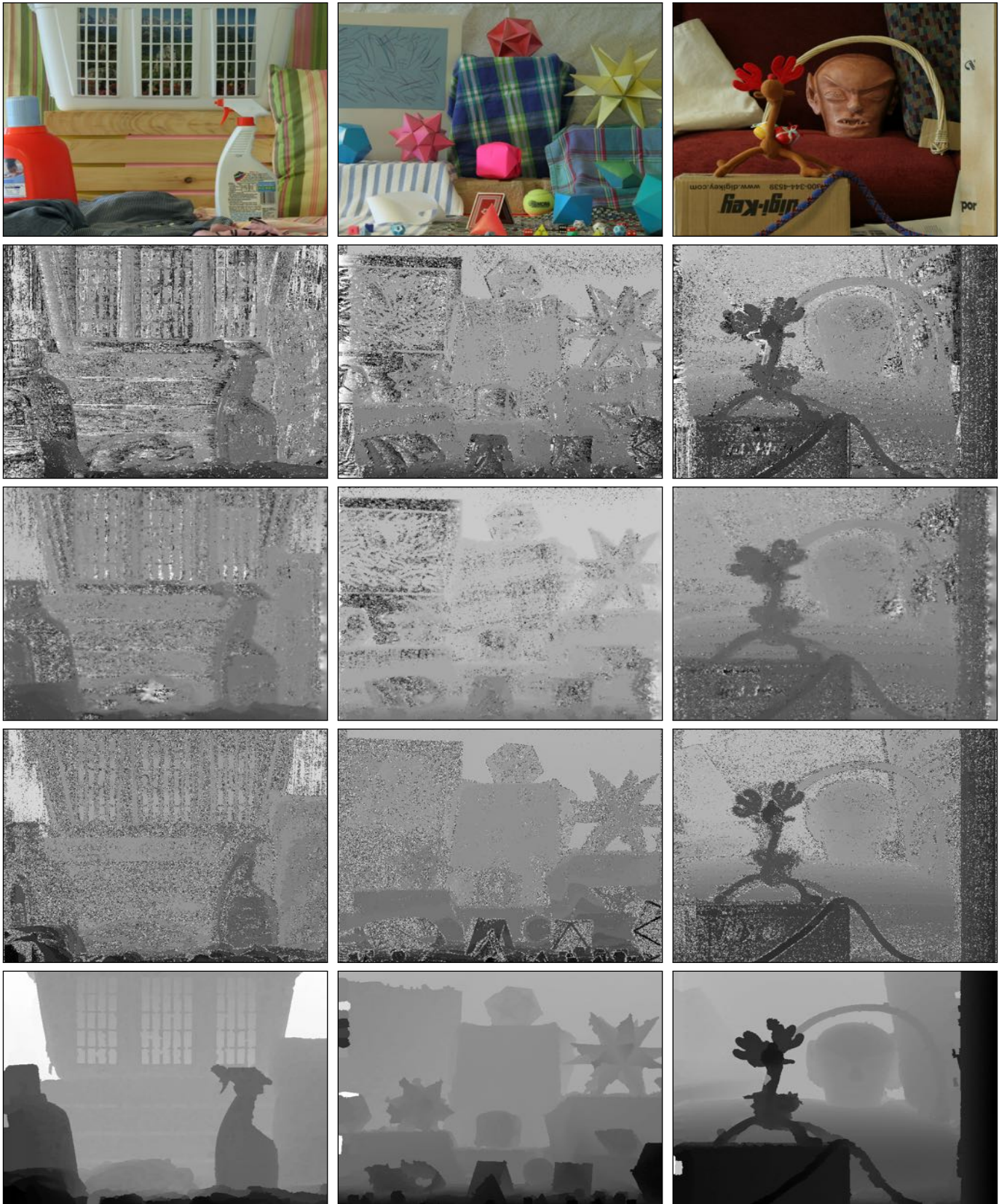
Figure 6: From top to bottom: the reference frame, the Best Map , the result of MKS , the result of Kalman T (temporal-only) and the result of Kalman ST . Images are automatically scaled in the range [0,255] , hence the gray levels changes from row to row. Full resolution images can be seen on line [1].
