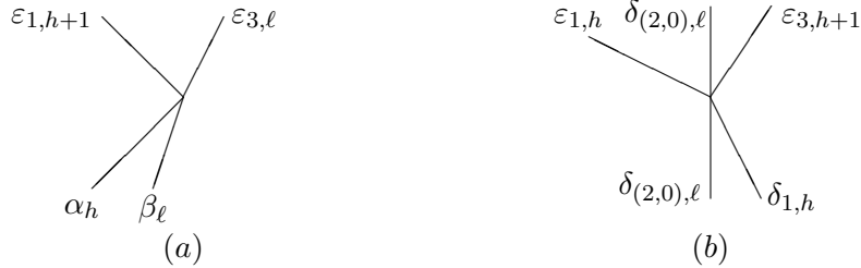
Figure 7: Interactions of waves; h and \ell denote generation orders. (a): interaction of 3-waves with h \geq \ell ; (b): interaction between a 1-wave and the (2,0)-wave solved by the Pseudo Accurate solver.
