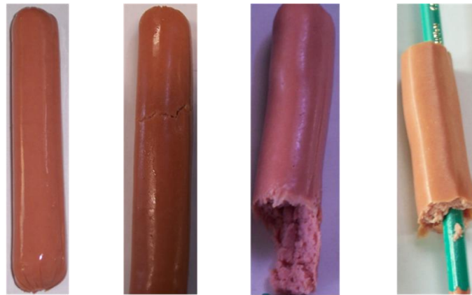
Figure 2 – Classification of the damage on fingers from left to right - scale of damage (1.2.3.4)
