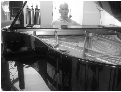
Figure 1: Setup for loudness estimation on the grand piano using a KEMAR mannequin.
