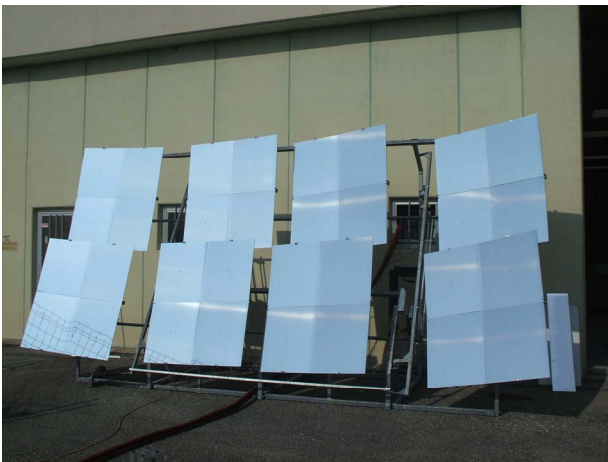
Figure 3. A Linear Mirror II device with eight mirrors.
