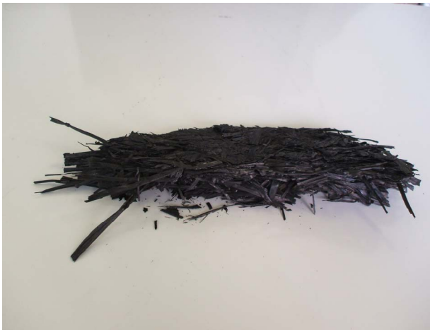
Figure 9. Material resulting from the torrefaction of hay.
